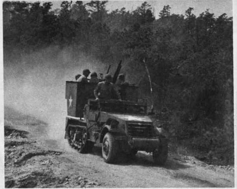
Square bucket of the M-15 covers the rear section of the half-track chassis and revolves with guns. The bucket is armored on three sides but is cut out in the rear. The chassis is the familiar M-3 half-track.
